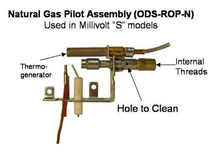
you have a log placement diagram for your log set. If you know that your gas logs are properly installed, then you can take a picture of the log placement for reference later. Insert the straw into the air intake hole pictured above and give it a puff of air. Also, blow air into the end of the pilot burner where the flame would be burning.
