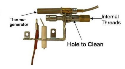
you have a log placement diagram for your log set. If you know that your gas logs are properly installed, then you can take a picture of the log placement for reference later. Insert the straw into the air intake hole pictured above and give it a puff of air. Also, blow air into the end of the pilot burner where the flame would be burning.
